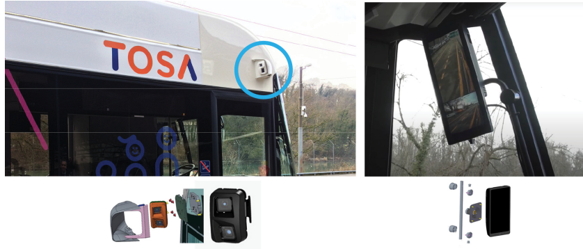
Camera affixed to exterior of vehicle; component & installation
