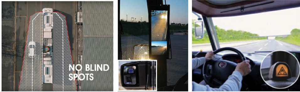
Blind spot elimination with Smart Vision CMS and BSIS+/MOIS+ ADAS
