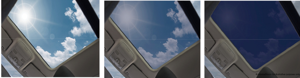
TOP: SPD Building Façade; Bottom: SPD Sunroof from ON to OFF in various dimming stages
