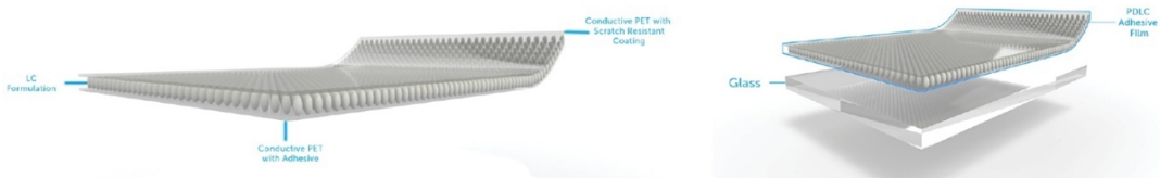
Liquid Crystal formulation coated between two sheets of conductive PET (ITO, nanosilver, etc) with adhesive and scratch-proof coating
