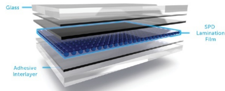
SPD Film laminated between two pieces of glass with adhesive interlayer
