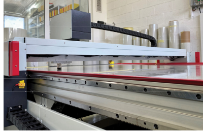
Laser Cutting Machine for Custom Size Film
