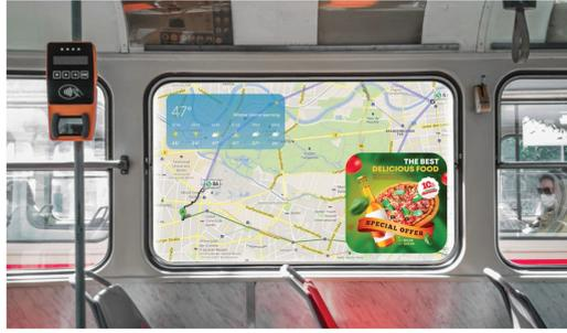
Representation of Acti-Vision on a train, or projection on combination PDLC and SPD
