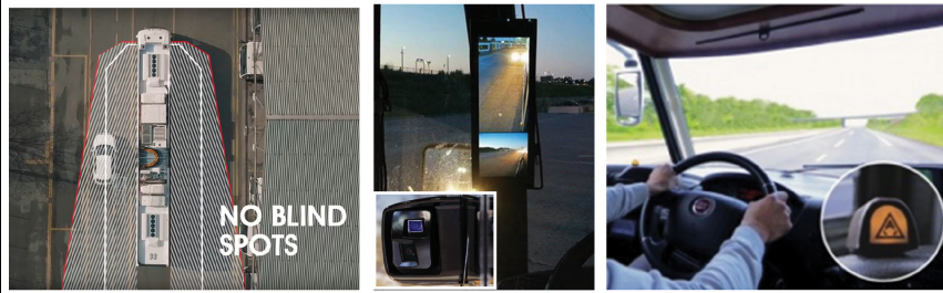
Blind spot elimination with Smart Vision CMS and BSIS+/MOIS+ ADAS
